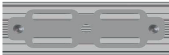
fixing plaque min n°2 every profile hole for screw \varnothing 3,5
